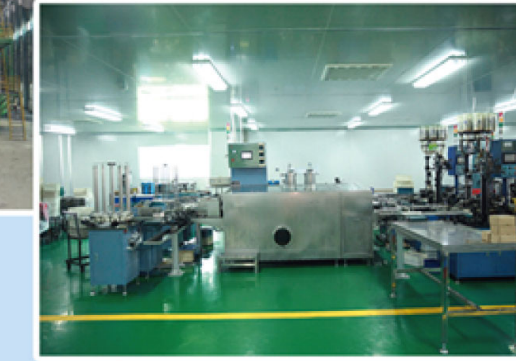
① Clean room: Automatic bearing assembly line
